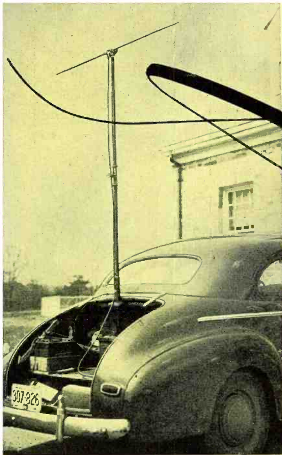
Rear view of car with trunk cover removed, showing how the antenna is mounted.
