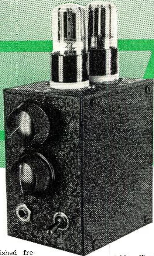
A metal box, 3" x 4" x 5", mounts all components.
